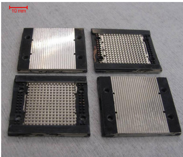
Fig. 7. Partly electroplated ABS bipolar plates.
